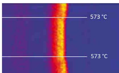
Figure 2: Phase transition from  $\alpha$  to  $\beta$ -Quartz at T=573°C
