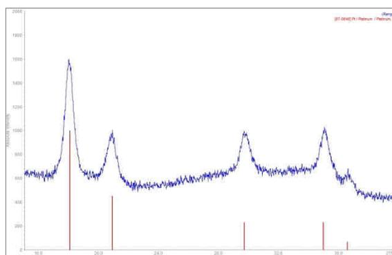
Figure 5: Pattern at RT with the red markers for Pt from the ICDD data base
